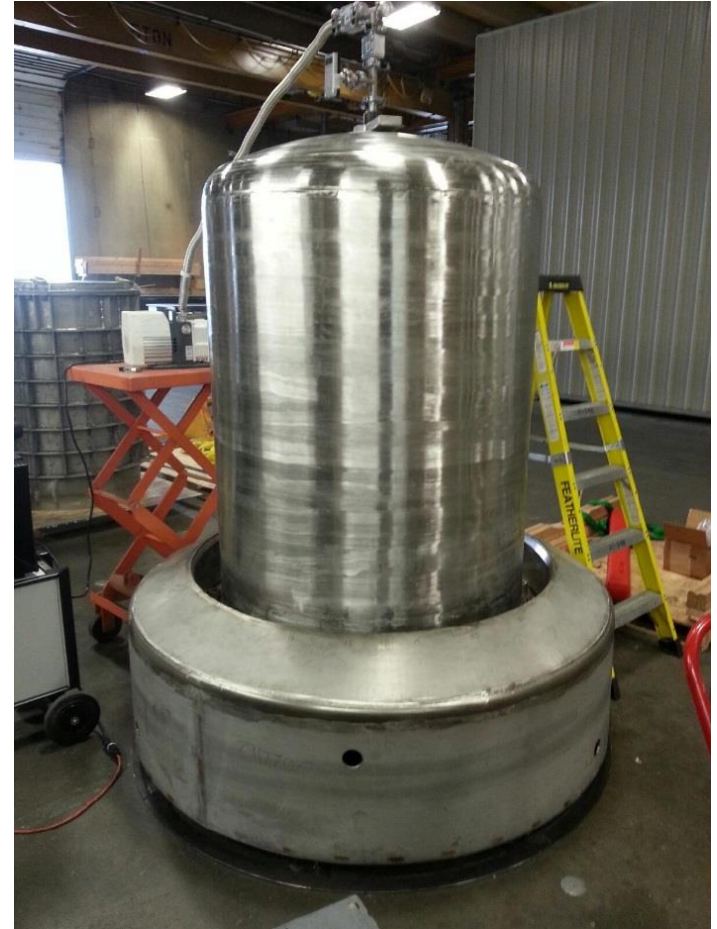
Assembled 435-B container ready for leak testing
