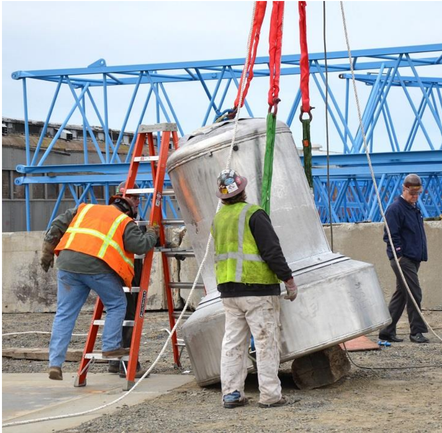
435-B Drop Testing of Test Unit
