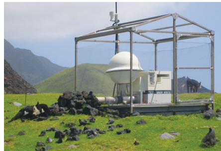
Figure 56. The Snow White air sampler as developed by Finland. Credit: CTBTO Preparatory Commission.
