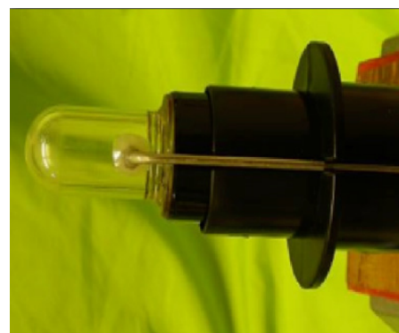
Figure 54. Example of a 4\text{ cm}^3 ( \sim 1\text{ cm} \times 4\text{ cm} ) plastic scintillator beta cell used in current \beta - \gamma detectors, designed to fit inside of a NaI detector well.
