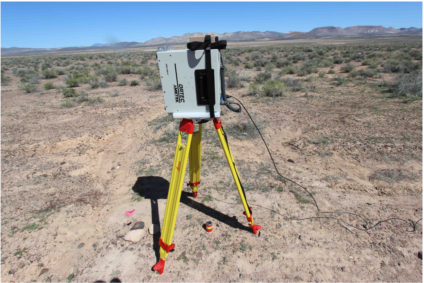
Figure 63. Field test of an OSIRIS spectrometer at the Nevada National Security Site. The small cylinder directly below the spectrometer contains a microcurie-strength fission-product source.
