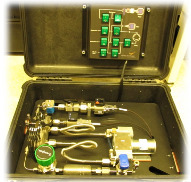
Figure 47. The calibration suitcase was developed to repeatedly and consistently deliver calibration gas to IMS stations.
