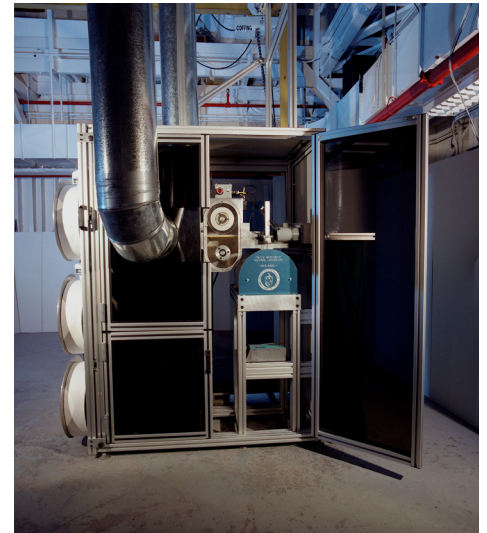
Figure 57. The RASA system as developed by the U.S., with a system footprint of 1m x 2m.
