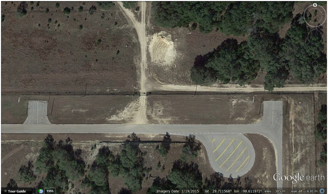
Appearance of facility, 2015. The large circle is a typical provision for turning long vehicles. The poles adjacent to the rectangular parking areas are possibly for lightning protection.
