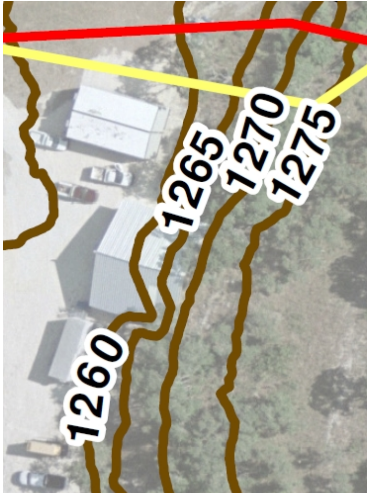
Detail from Figure 3 above. Note that natural contour increases by approximately 10 feet from the front to the back of the building.
