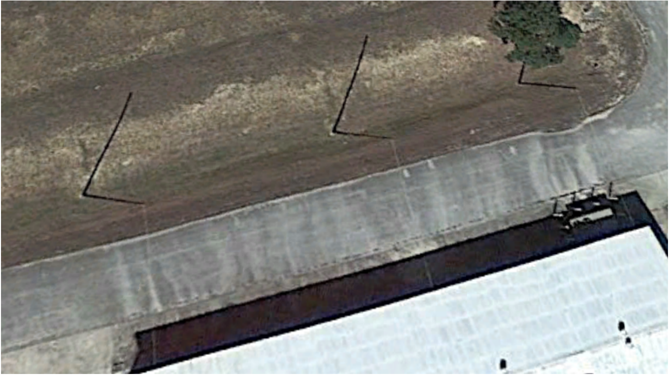
Close-up of masts on north side of building. Faint lines, possibly overhead ground wires, extend from the masts toward the building.
