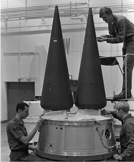
Fig. 2. This shows two low-drag RVs being placed on a Minuteman III missile, which can carry three RVs. (Source: US Air Force).
