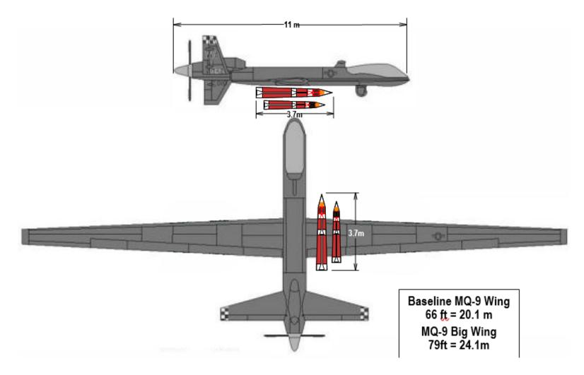
The workhorse MQ-9 "Reaper" from General Atomics Aeronautical Systems Inc. The "Big Wing" version is stated to have an endurance of almost 24 hours at 500 km from its operating base, patrolling at an altitude of about 35,000 feet.
