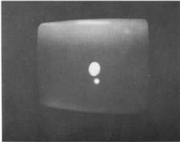
Fig. 3. Video image of the eye as observed on the slave monitor. The large disk is the pupil observed in light retro-reflected from the retina. The bright spot is a de-magnified virtual image of the illumination source formed by specular reflection from the curved front surface of the cornea.
