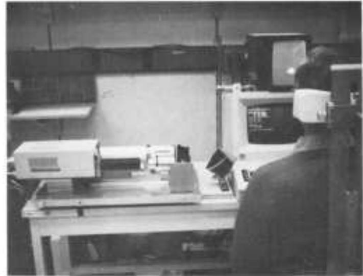
Fig. 4. Photograph of the eyetracker. The illumination system is inside the white tube in the background. The TV camera is at the left. The gimbaled aiming mirror is just to the left of the display terminal.
