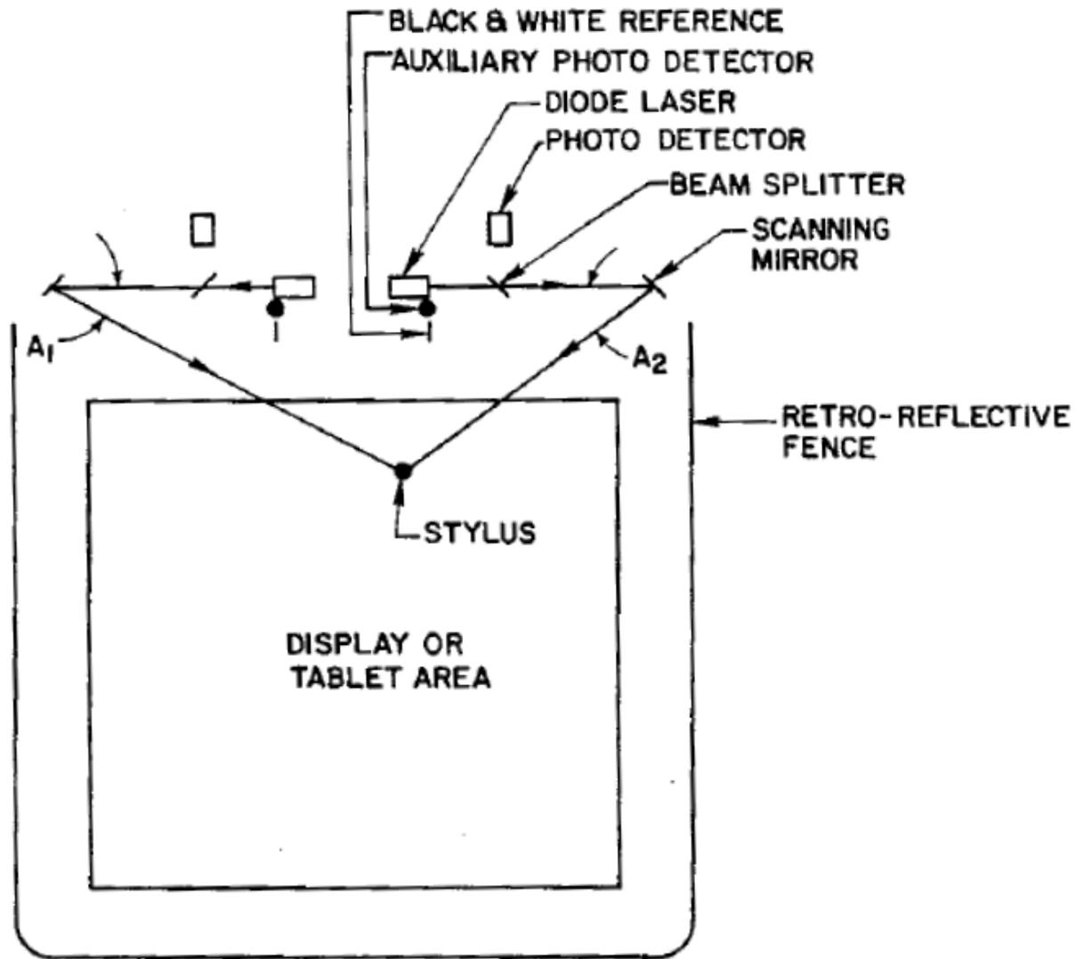
FIGURE 1: Device geometry and parts arrangement.
