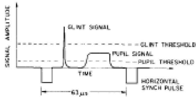
Fig. 5. Video signal for a raster line which crosses the glint and then the pupil. Typical threshold levels are indicated (dashed lines) as well as the horizontal sync pulses.
