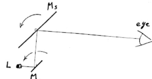
Fig. 2. In ROLED display, use of auxiliary mirror  $M_a$  to take light at constant angle from the LEDs as the main scanning mirror  $M_s$  rotates. This allows use of LEDs with smaller emission solid angle.
