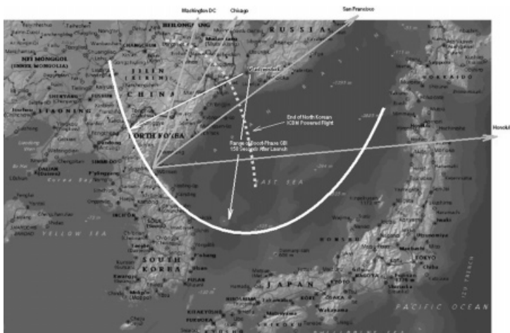
FIGURE 12. Engagement Region of Russian-U.S. 100-Second Burn-Time Ground-Based Interceptor Against North Korean 250-Second Burn-Time ICBM
