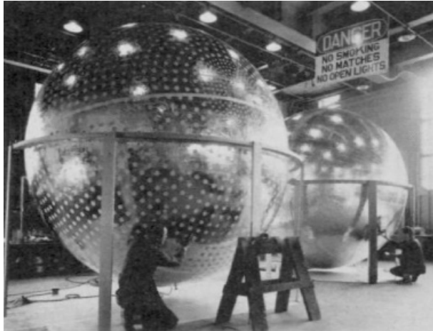
FIGURE 6. Figure 8-1 of “Countermeasures,” photograph of NASA Air Density Explorer balloons, first launched in 1961
