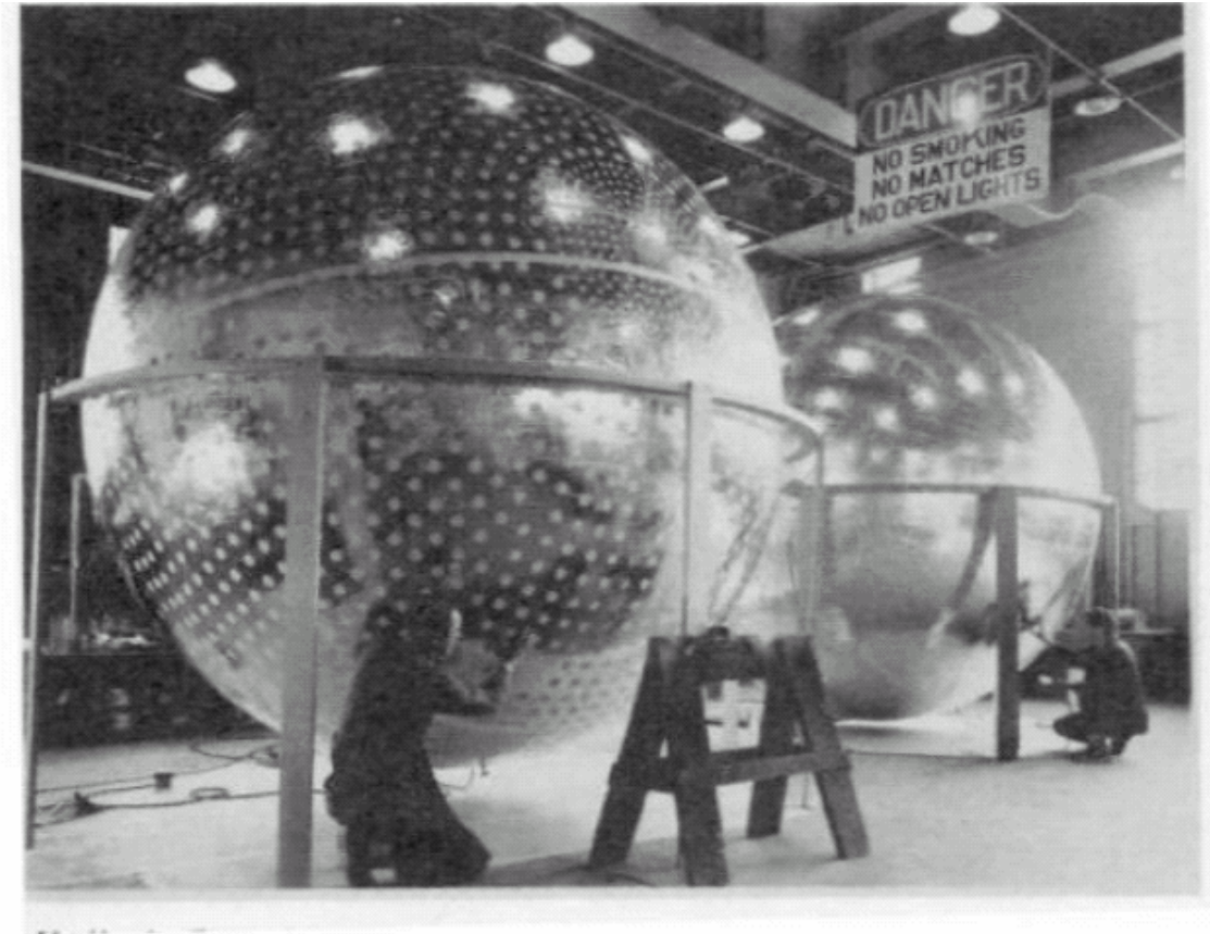
Figure 8-1. A photograph of one of the NASA Air Density Explorer inflatable balloon satellites.
