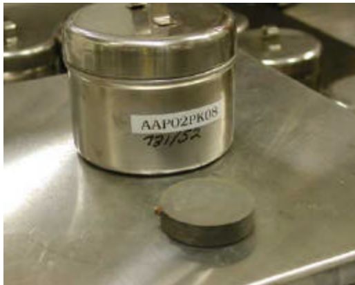
First LANL Pu-238 spiked delta-Pu casting, May 2002 (Friebert, Olivias, et al)
