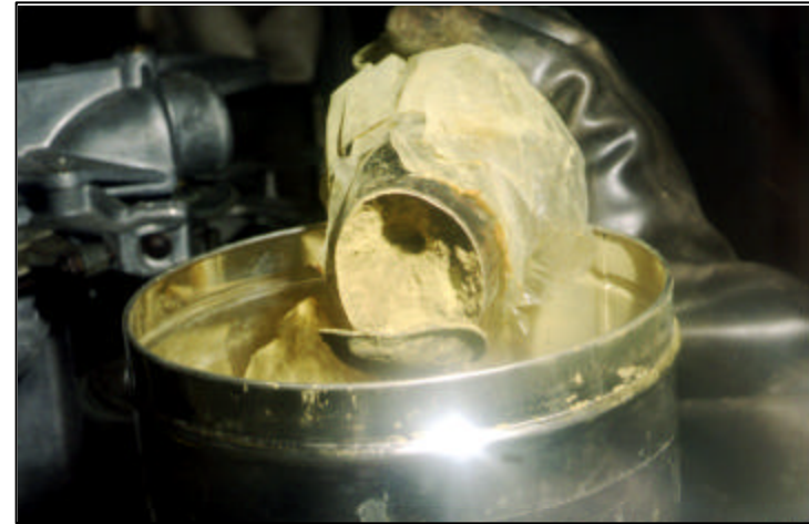
Corrosion of Metallic Pu in a defective Storage Container (Haschke and Martz, Plutonium Storage 1998)
