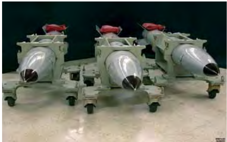
Figure A-2-2. B61 bombs represent some of the oldest designs in the active nuclear weapons stockpile. Recent alterations continue the process of extending service lifetime by refurbishing spin rocket motors and some canned sub-assemblies.
