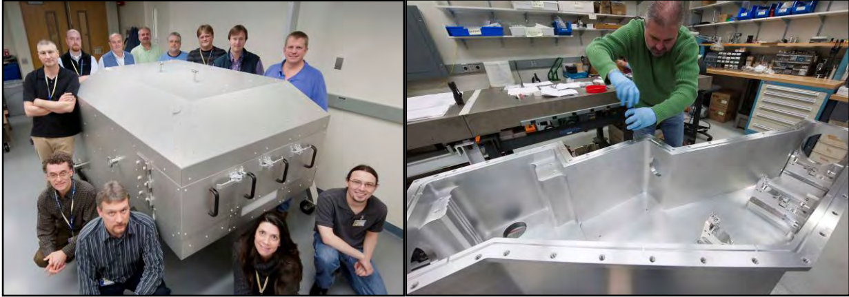
Figure A-5-6. The Magnetic Recoil Spectrometer that has been delivered to LLNL for installation on the NIF. It will measure the neutron energy spectrum that will be used to determine the areal density of implosions during the ignition campaigns. Left panel: assembled diagnostic weighing 9000 lbs, shown with team members from Massachusetts Institute of Technology and LLE. Right panel: interior of the diagnostic.
