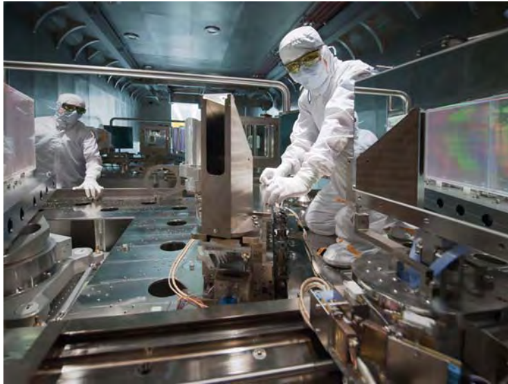
Figure A-5-10. A view inside the OMEGA EP Grating Compression Chamber at the University of Rochester. The chamber houses the optics including the tiled grating assemblies that can compress two of the EP beams to short pulse (1 to 100 picoseconds).
