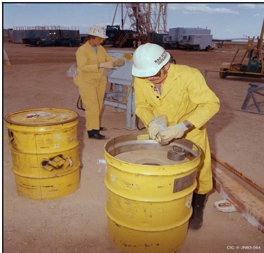
Figure 3-6. Packaging drillback samples for laboratory analysis. Photo courtesy Los Alamos National Laboratory.
