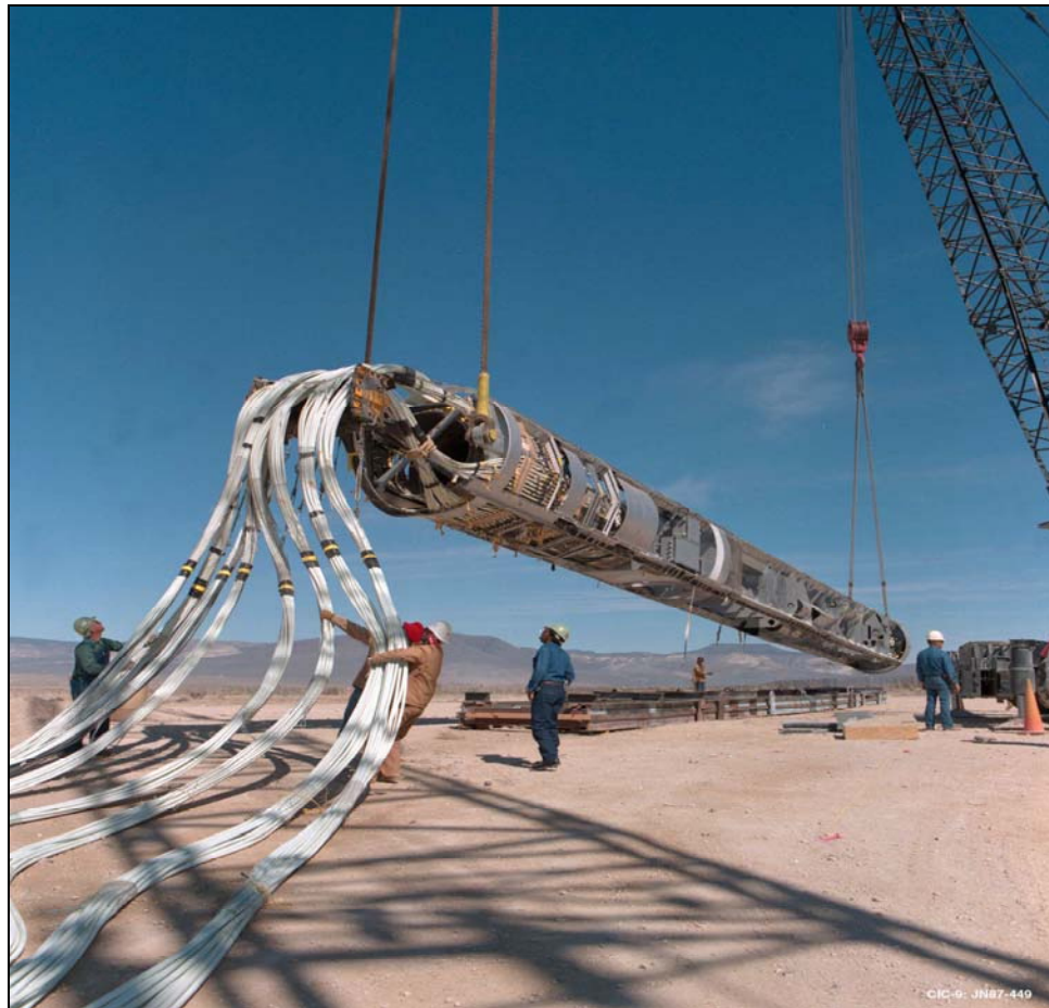
Figure 3-1. Setting up test rack at the Nevada Test Site. Note bundles of cabling attached to rack. Photo Courtesy Los Alamos National Laboratory.
