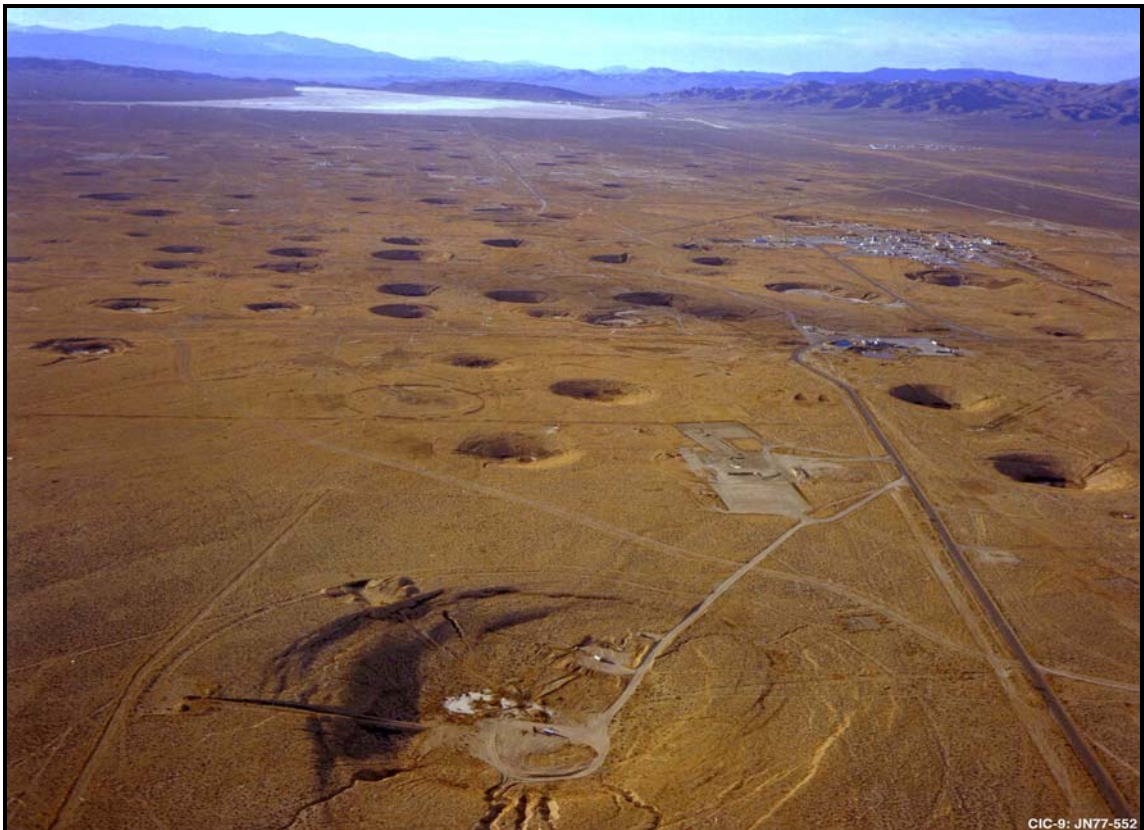
Figure 3-8. Aerial photo of subsidence craters at the Nevada Test Site. Photo courtesy Los Alamos National Laboratory.
