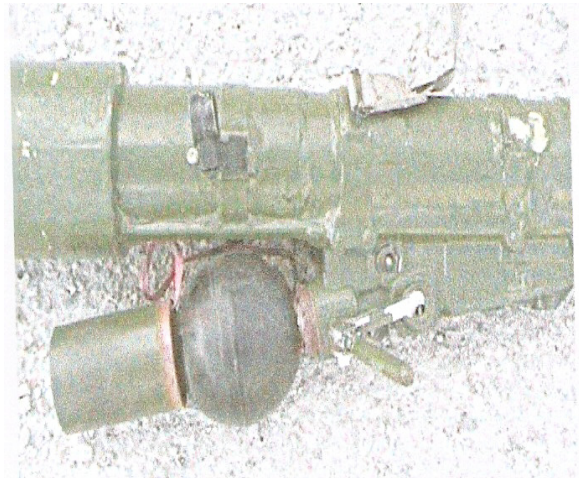
Close-up of battery/coolant unit on SA-18 missile found in Somalia
