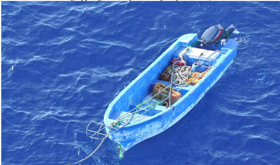
Typical pirate attack skiffs with 60HP Yamaha outboard engine, ladder with welded bow, grappling hook, ropes, and spare fuel (2010)
