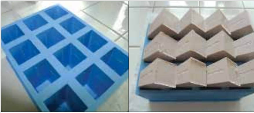
LEFT: This is the prototype mold that will be used to see if molding explosives can be a viable option to create explosive charges. The mold cuts down on production costs and time as it preforms the end product into its exact size and weight required by the deminers, instead of the current method which involves pouring the explosives into a pan and cutting them into "brownies." RIGHT: This is the first test run of the new explosive molding system using inert resin as a casting agent instead of live explosives. Initial tests showed good results as the charges were released from the mold easily and still retained a lot of the detail within the mold and its engravings.
