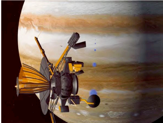
Figure 1. Galileo spacecraft in orbit about Jupiter. One of the two GPHS-RTGs shown at the top. (NASA/JPL)
