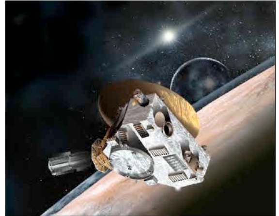
Figure 4. New Horizons spacecraft shown flying by Pluto with satellite Charon in the background. The single GPHS-RTG is shown mounted on the left side of the spacecraft. (JHU/APL and SwRI)
