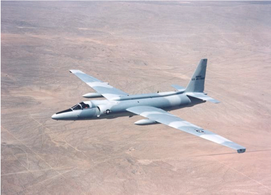
The U-2C had fluted inlets to accommodate increased airflow to the J75 engine and a dorsal spine housing additional equipment. Note the 100-gallon slipper tanks on each wing. (Lockheed Martin)
