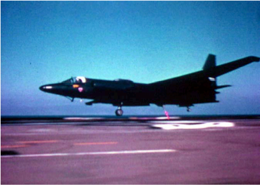
U-2 pilot attempts to snag the arresting cable during landing aboard the Kitty Hawk . (Lockheed Martin)
