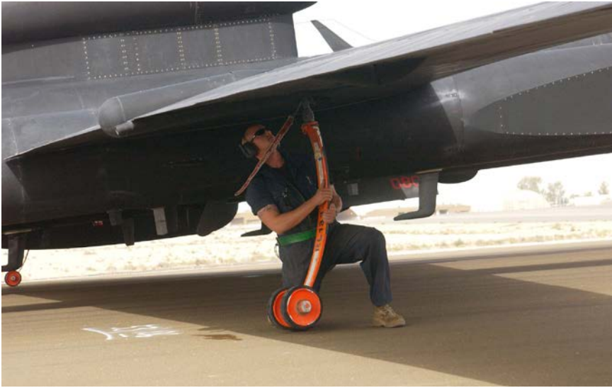
Senior Airman Jordan Mihm installs an outrigger pogo on a U-2R. (U.S. Air Force)
