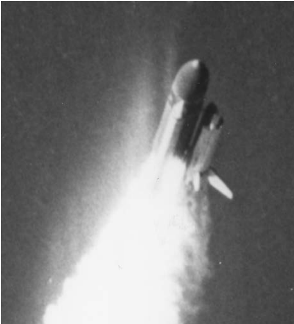
U-2 imagery of Space Shuttle Atlantis taken on May 4, 1989. The resolution was insufficient for determining the source of debris from the SRB nose caps. (U.S. Air Force)
