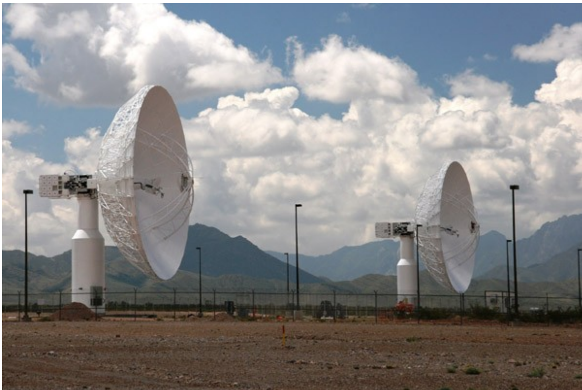
Two of the new 18-meter Ka band dishes installed at the White Sands Test Facility in New Mexico. Credit: NASA
