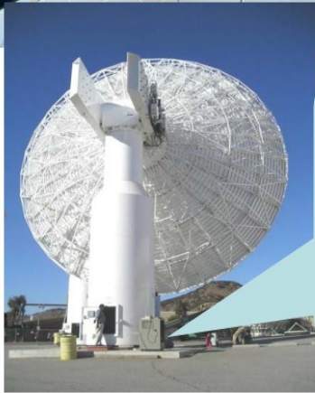
LRO Reflector Mounted on the First SDO Pedestal During Acceptance Testing at the Vendor Facility
